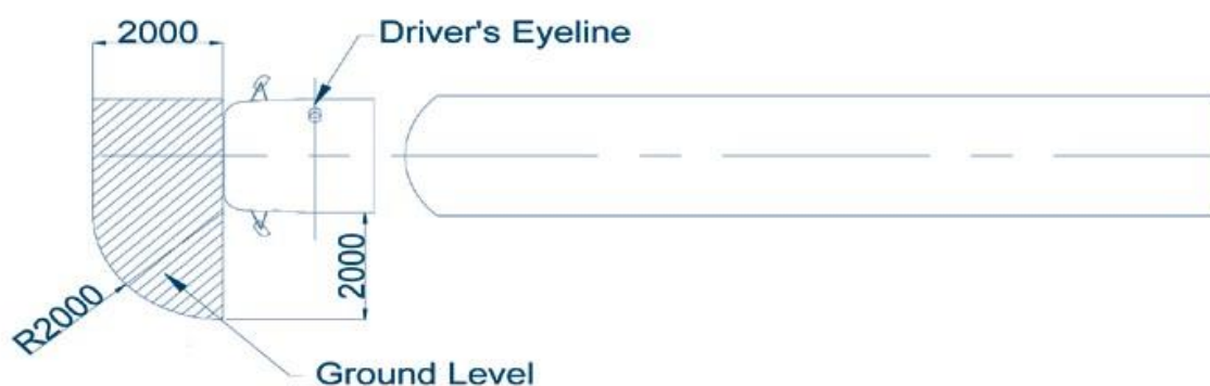
Figure 2: Field of vision of Class VI front mirror (All dimensions in millimetres).
